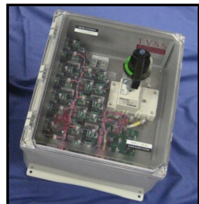
TSrc300 With Fused Disconnect & NEMA 4X Enclosure with Clear Hinged Cover
