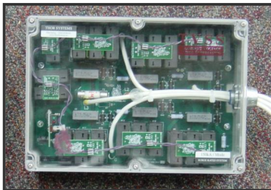
TSn150 with LEVEL 1 MONITORING Visible Through Transparent Cover of NEMA 4X Enclosure
