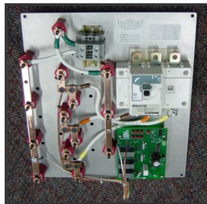
TSrc300 BACKPAN Depicts "StakTraks™" Low Impedance Parallel, All Copper Buss Structure
