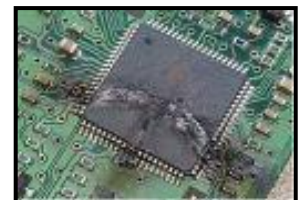
Failed Microchip (Inexpensive Components Cause Large Financial Losses)
