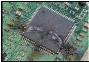
Failed Microchip (Inexpensive Components Cause Large Financial Losses)
