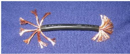
#6 AWG “Rope-Lay” Wire 259 Strands of #30 AWG (.010" dia.) (7 twisted groups of 37 strands/group) VS. #6 AWG THW/THHN (19 Strands)
